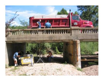
Figure 4-1 – Load Test with H20 Truck
