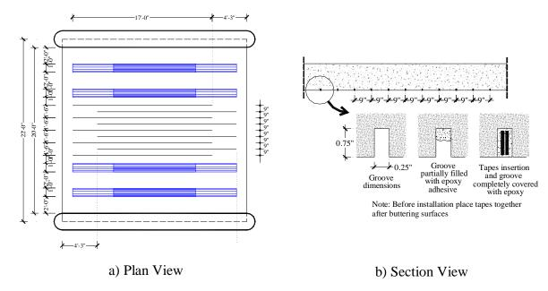
Figure 3-4 – Strengthening with NSM Bars and CFRP Laminate on Span 2
