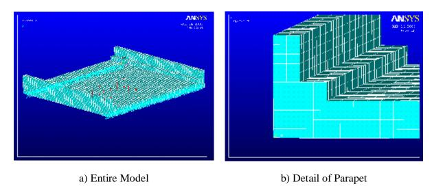
Figure 6-1 – FEM Model Geometry
