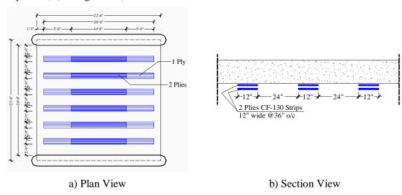
Figure 3-2 – Strengthening with Laminates on Span 1 and 3
