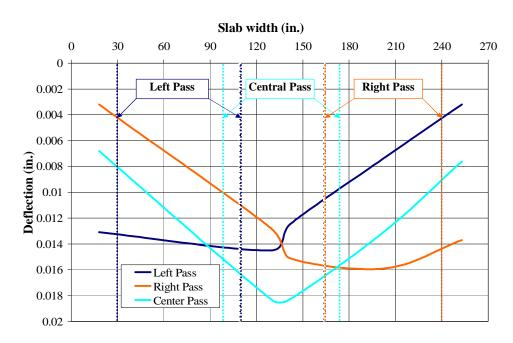
Figure 4-4 – Mid Span Deflection in the Transverse Direction, Stop No.3
