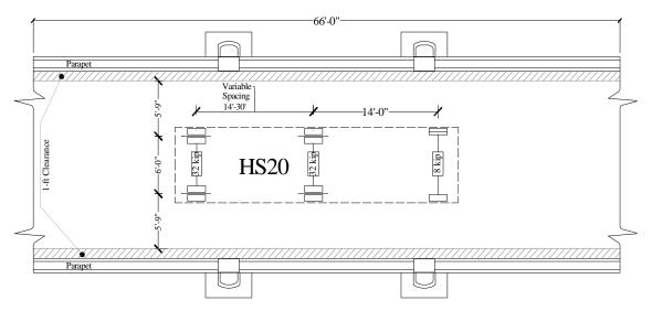
Figure 2-2 - Truck Load and Truck Lanes
